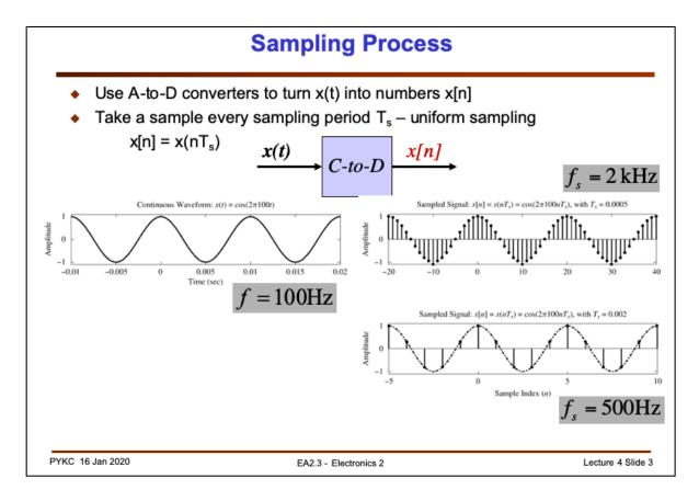
Again you should be familiar with the sampling process already. The important point to note here is that we currently only consider UNIFORM SAMPLING, meaning that we take a sample of the signal x(t) at regular intervals of period Ts, where 1/Ts = sampling frequency.
