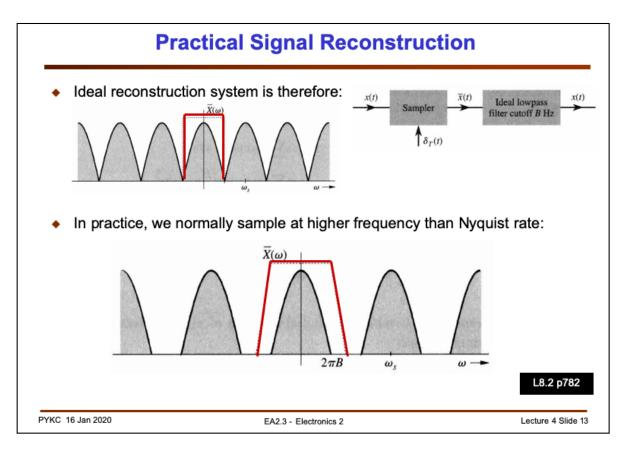
So in practice, we DON'T use the sinc function for reconstruction. Instead we sample the signal at highest than Nyquist rate (i.e. fs >> 2 fmax), introducing the gaps, and therefore allow us to use much gentle filter with less abrupt changes in the spectral domain.
