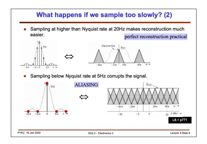
If we sample at higher than 10 Hz, then the effect is to push apart the triangles as shown, with gaps between them in the frequency spectrum. This makes reconstruction much easier — we can use a lowpass filter that is easy and economical to implement as shown. This is NORMALLY what is being done. We usually sample the signal with  $fs \ge 4 x$  fmax as shown here in order to make reconstruction easy.
