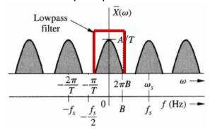
This is only possible if the shaded parts do not overlap. This means that fs must be more than TWICE that of B.
