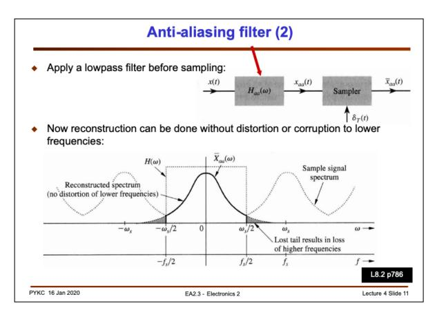
In order to avoid such corrupt, we must always apply a lowpass filter to the continuous time signal BEFORE sampling is performed. This cuts off the energy beyond fs/2, and therefore avoid corrupting the original signal spectrum (and hence the original signal) because now there is NO aliasing or spectral folding.
