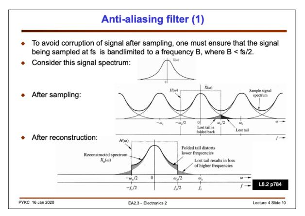
The consequence of this theorem is that, in order to avoid corruption of the information (signal), we MUST limit the bandwidth of the signal, BEFORE sampling taking place. In the diagram here, the original signal has very small energy at the tail of the spectrum as shown.
