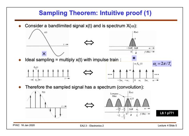
We can mathematically prove what happens to a signal when we sample it in both the time domain and the frequency domain, hence derive the sampling theorem.
